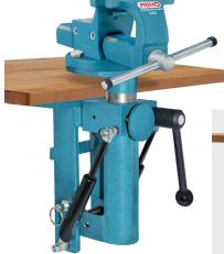
After loosening the left safety clamping lever the vice can be easily adjusted into the desired working position.
